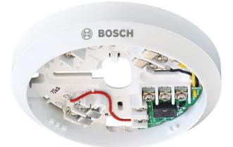
The MSR 320 Conventional Detector Base with Relay can be used to mount detectors from the 320 Series. The MSR 320 is provided with an integrated relay that has NO/C/NC contacts for switching applications (e. g. dampers, door holders, etc.).
